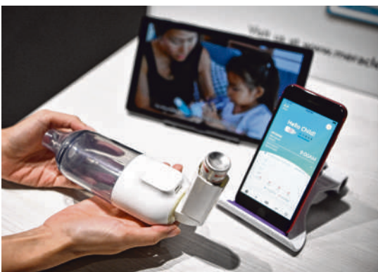
The Whizz provides users with visual feedback that reinforces the correct inhalation of asthma medication. ST PHOTO: ARIFFIN JAMAR
